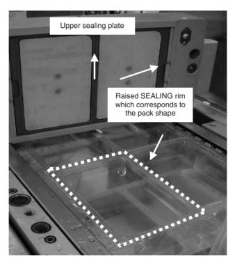
Fig. 10.10 Top web heat sealing on thermoform fill seal machine. (Courtesy of Multivac.)
