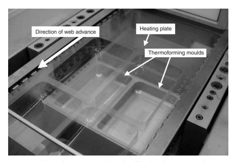
Fig. 10.9 Base web thermoforming section on thermoform fill seal machine. (Courtesy of Multivac.)
