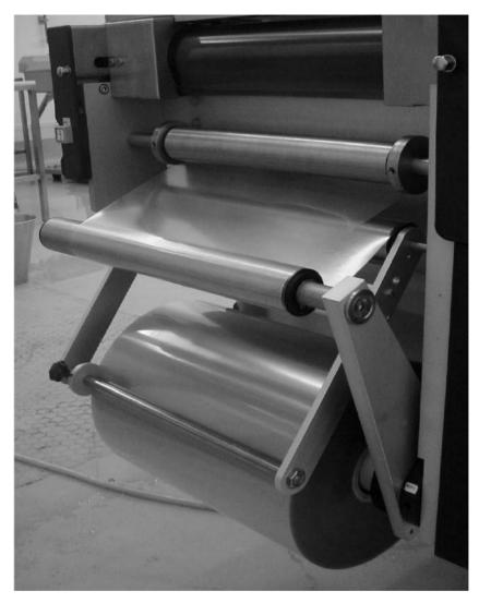
Fig. 10.8 Lower web unwind and infeed section on thermoform fill seal machine. (Courtesy of Multivac.)
