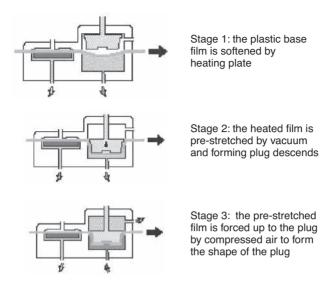
Fig. 10.5 Thermoformed tray produced by plug assisted positive forming. (Courtesy of Multivac.)
