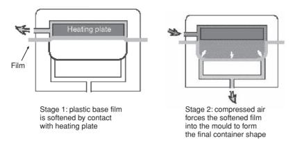
Fig. 10.3 Thermoformed base tray produced by negative forming method. (Courtesy of Multivac.)
