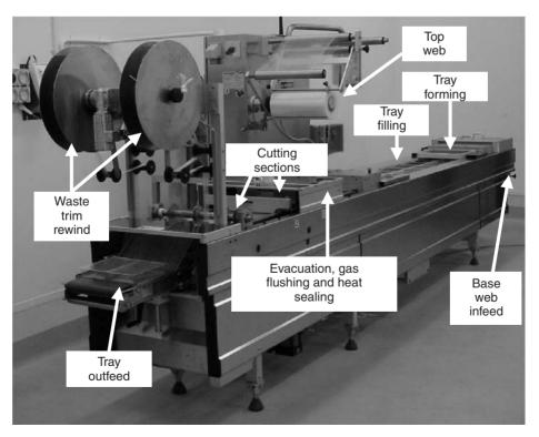
Fig. 10.7 Thermoform fill seal machine. (Courtesy of Multivac.)
