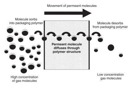
Fig. 10.1 Permeability model for gases and vapours permeating through a plastic packaging film.
