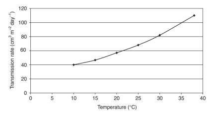
**Fig. 10.2** The effect of temperature on the transmission rate of  $CO_2$  in  $25\mu$  PET film measured at 0% RH and 100%  $CO_2$ .
