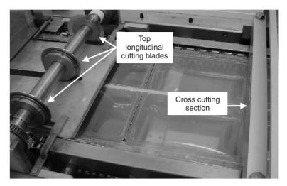
Fig. 10.11 Cutting section on thermoform fill seal machine. (Courtesy of Multivac.)
