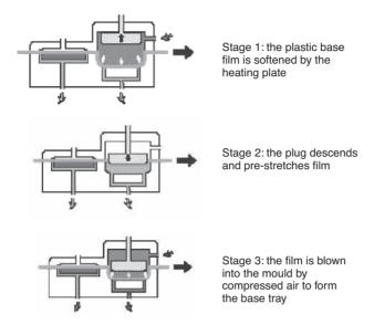
**Fig. 10.4** Thermoformed base tray produced by the plug assisted negative forming method. (Courtesy of Multivac.)
